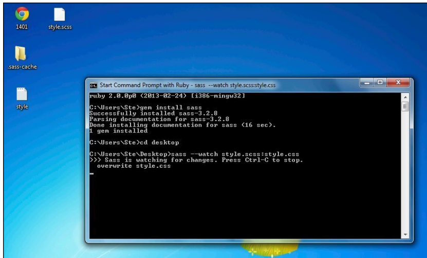
Figure 14-6 Tell Sass to watch the .scss file for any changes and then compile this code into a standard .css file (which has been automatically generated).
