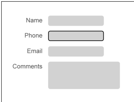
Figure 16-4 When a label element is hovered, the input element with an id value matching the label element's for value is given a black border.
