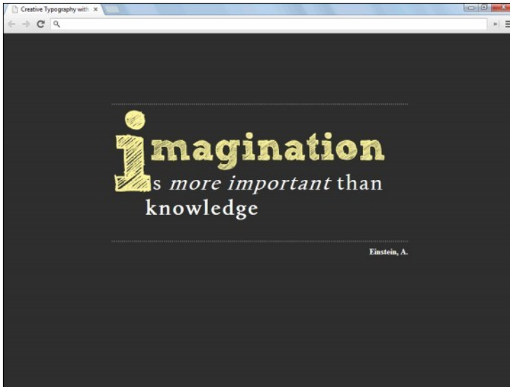
Figure 13-5 The first letter has been maneuvered into place and now covers up the i from the word is so it can act as its replacement.
