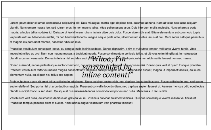
Figure 11-7 The content spans across all three columns and all three rows, and the blockquote element is currently dumped on top.
